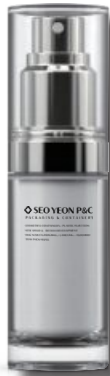
SY17-J7-E20 20ml 32Ø X 114mm NECK 20Ø OVER CAP : SAN SHOULDER : ABS INNER BOTTLE : PP OUTER BOTTLE : SAN
